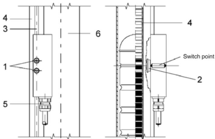
Mounting the magnetic switch (model MA)
