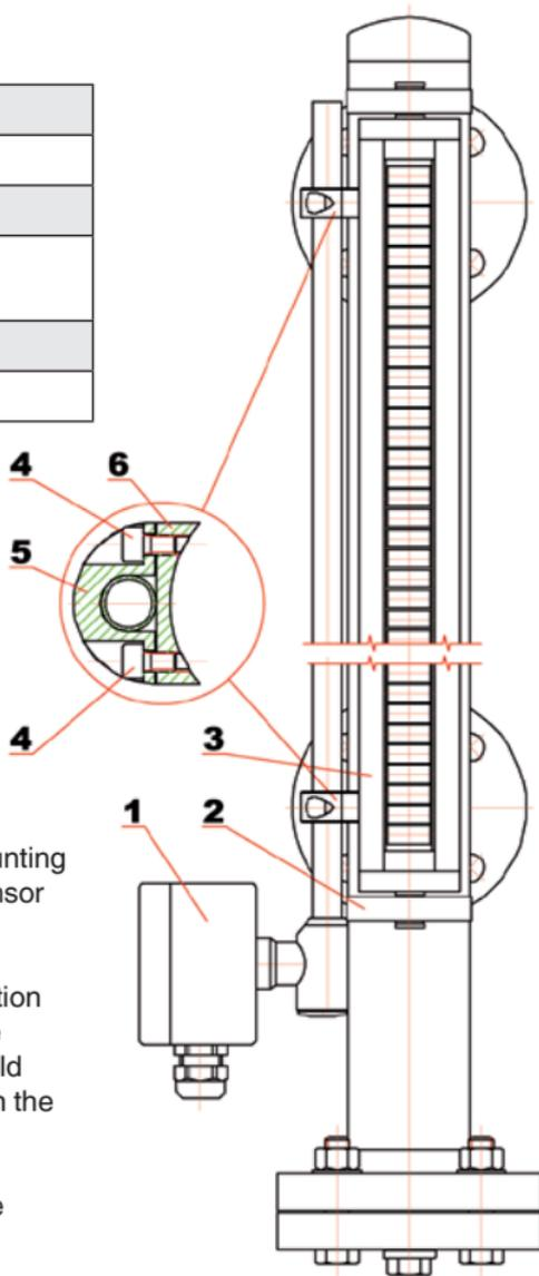
Use the tightening strap or mounting clamp (pos. 5) to attach the sensor MG ... to the bypass tube.
