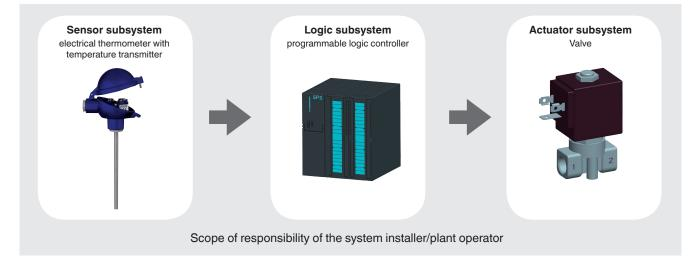
An electrical thermometer with models T32.1S temperature transmitter (head mounting version) and T32.3S (rail mounting version) can be used by the plant operator as a sensor subsystem of a safety instrumented system.
