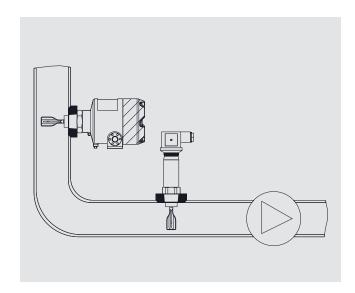
To ensure that a pump does not run dry, there must be sufficient liquid in the intake pipe. The vibrating level switch can detect this and thereby prevent damage to the pump. Since the tuning fork only protrudes 38 mm [1.5 in] into the pipeline, it can be used to measure in small diameter pipelines.
