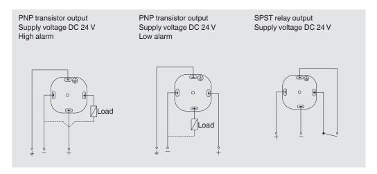
TLS-HM Circular connector M12 x 1, 4-pin
