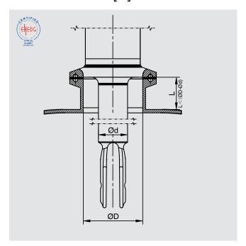
Sensors inserted in tanks should be flush with the inside of the tank wall. If, for technical reasons, there is a dead space, it must be ensured that the spray jet from the cleaning appliance can reach all surfaces. To fulfil the EHEDG cleaning criteria, the maximum length of the tank nozzle,  $L_{\text{max}}$ , should be taken into account.
