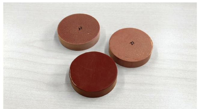
Colour changes in cast resin samples as a result of decomposition products in SF 6 gas
