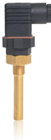
The TFS35 is a bimetal temperature switch and can be designed as a normally closed or normally open contact. Due to its high transmissive electrical switching power, it can be installed into a load circuit without an interposing relay. This means that neither an additional voltage supply nor a signal input on control electronics is necessary.
