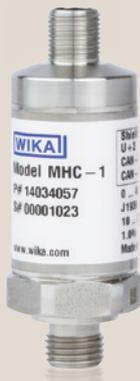
The MHC-1 combines the characteristics that all pressure sensors of the MH product line feature with a CAN signal interface. This is controlled by the SAE J1939 or CANopen® communications protocols. The MHC-1 ensures optimal sensor connection in CAN systems with simple installation and individual CAN configuration.
