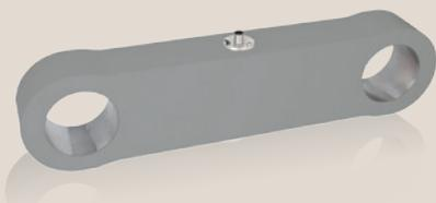
The F7301 is a tension link for static and dynamic tensile force measurement directly in the flow of forces. It is made from high-strength fine-grain structural steel or stainless steel. State-of-the-art welded-in thin-film elements provide the force measurement. As an OEM product, the F7301 is designed and manufactured specifically to customer requirements. Therefore, a multiplicity of product execution can be provided in terms of nominal load, geometry and signal output.
