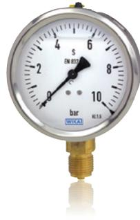
The model 213.53 Bourdon tube pressure gauge in a stainless steel case is suitable for the pressure indication at increased media temperatures. The liquid filling ensures a high degree of indication accuracy with dynamic pressure spikes and vibrations.
